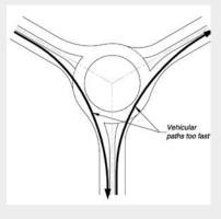
In situations involving a large angle between legs, it is desirable to realign one or more legs to achieve a more perpendicular condition. Large angles make it difficult to provide adequate deflection and may result in fast vehicle speeds, particularly for rightturning movements.
