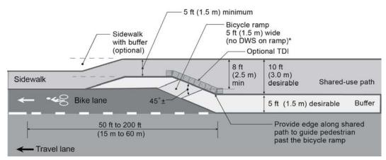
\*DWSs are no longer recommended on bicycle ramps. If desired, optional TDIs can be used to delineate the desired path for pedestrians near the ramp. See FHWA (12).
