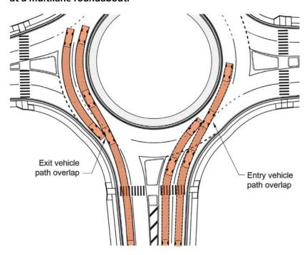
Exhibit 9.24. Examples of poor vehicle path alignment at a multilane roundabout.
