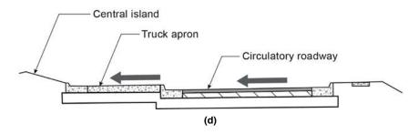
Exhibit 11.10. Example of circulatory roadway sloped inward to central island with sloped catch basin grate.
