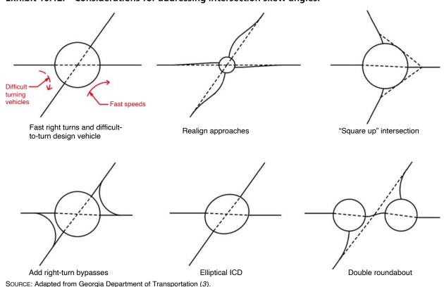
guide roundabout approach horizontal alignments, including the transition length and range of horizontal curve radii leading from the approach to the roundabout entry. Accommodating the design vehicle can also influence roundabout approach alignment and entry.
