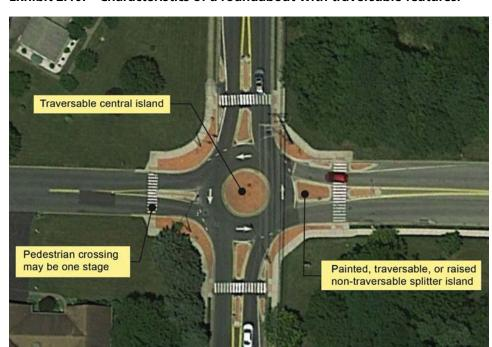
Exhibit 2.10. Characteristics of a roundabout with traversable features.
