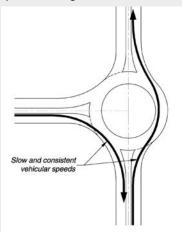
Perpendicular approach angles generally provide slow and consistent speeds when combined with other appropriately sized design features. Achieving acceptable fastest path speeds is often easier to accomplish with a perpendicular approach angle than with a skew.
