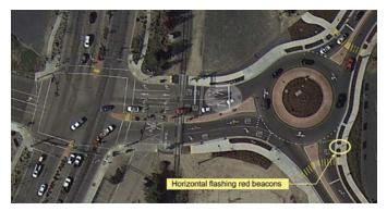
NOTE: Railroad gates are located only at the at-grade railroad crossing. Supplemental horizontal flashing red beacons are located on the roundabout leg in the lower right corner of the image. LOCATION: N Reed Avenue/W North Avenue, Reedley, California. SOURCE: Google Earth.
