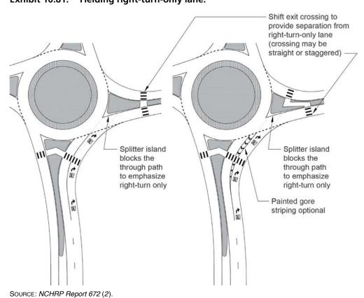
The exhibits are conceptual only to reflect this bypass type. The view angle for a driver in the right-turn-only lane may be insufficient, depending on overall roundabout geometry. In addition, the pedestrian crossing on the exit needs to be located farther from the end of the right-turn-only lane to provide drivers with sufficient time to react to and stop for pedestrians.
