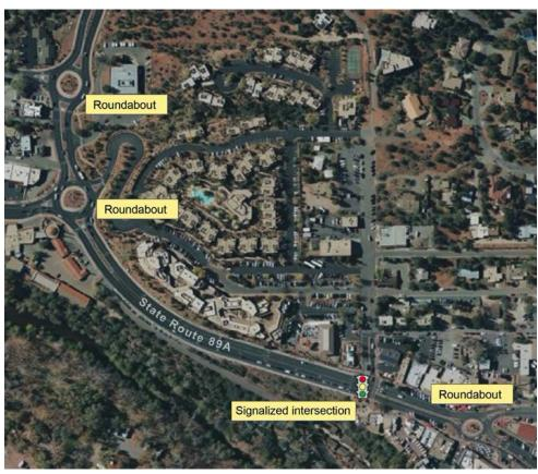
Exhibit 3.8. Example of mixing roundabouts with a signalized intersection.
