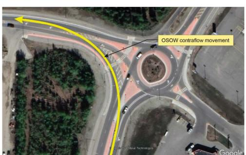
Exhibit 10.41. Example of OSOW contraflow movement using a bypass lane.
