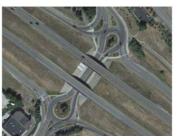
Exhibit 3.6. Example of roundabout at interchange ramp terminal intersection.
