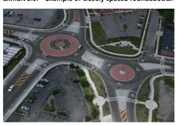
Exhibit 3.9. Example of closely spaced roundabouts.
