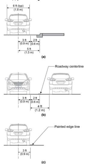
Limited relief vertical curb lips, rolled curbs, and other curb and gutter forms that are less concerning for a driver could lead to actual driving paths that infringe on the assumed buffer of 2 ft (0.6 m) to the curb face.
