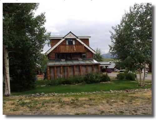
The sun space addition to this home was renovated. The glazing was replaced with walls and conventional window openings.
