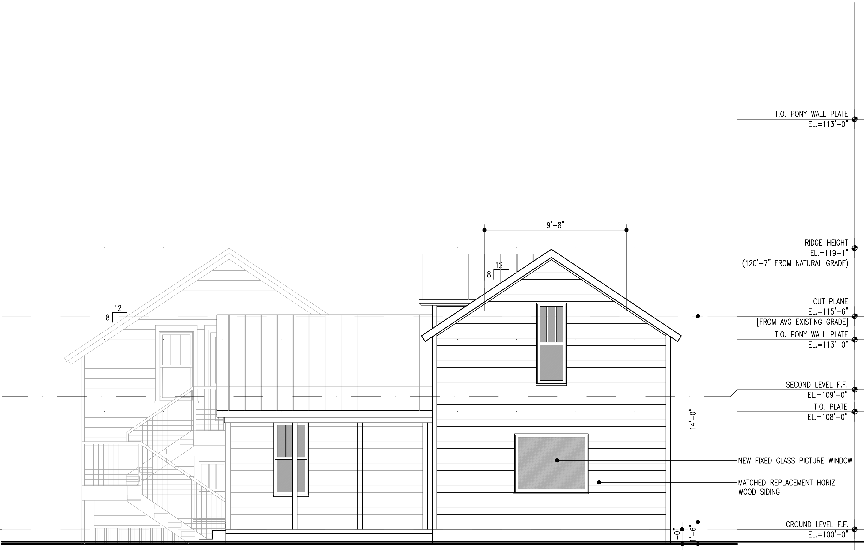
02 PROPOSED NORTH ELEVATION SCALE: 1/4"=1'-0"
